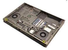
12. Remove the two screws at the rear of the computer.
