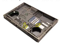
12. Remove the antennas from the routing channels.
