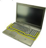
$\textbf{5.} \quad \text{Lift up to remove the keyboard trim from the unit.}$
