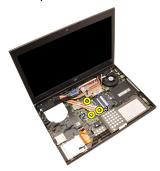
11. Lift up the CPU heatsink and remove from the system.
