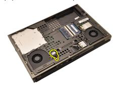
**6.** Remove the coin—cell battery from the system.
