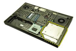
6. Remove the screws securing the optical drive bracket.
