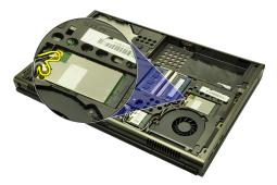
5. Remove the screw securing the WWAN in place.
