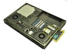
**8.** Flex the hard drive bracket outward and press the hard drive upwards from the bottom.
