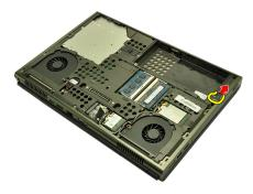
7. Remove the hard drive bracket from the system.
