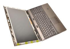
5. Remove the screws on the right side securing the display panel in place.
