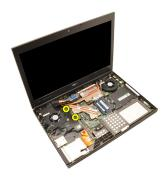
11. Lift the right edge of the I/O board upwards to disengage the connector and remove from the system.
