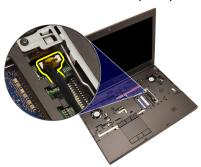
**16.** Disconnect the fingerprint reader cable.
