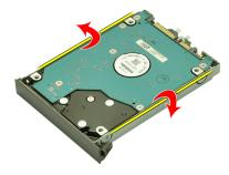
9. Remove the hard drive from the hard drive bracket.
