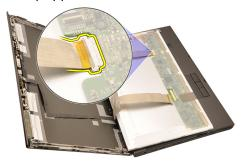
9. Remove the display panel from the display assembly.
