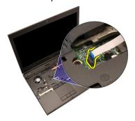
15. Disconnect the Radio Frequency Identification (RFID) cable.
