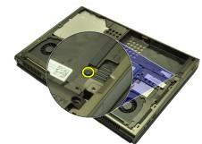
6. Slide the hard drive release latch into the unlock position.
