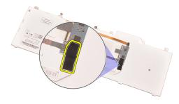
9. Disconnect the keyboard data cable from the back of the keyboard.
