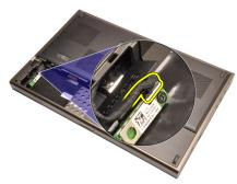
5. Remove the single screw securing the Bluetooth card in place.
