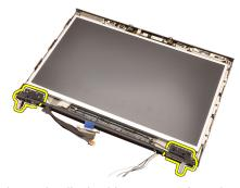
**15.** Release the display hinge towers from the cables and remove the hinge towers.
