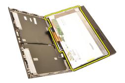
11. Remove the screws securing the display bracket to the display panel.
