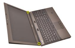
4. Remove the screws securing the display bezel in place.
