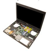
**14.** Lift up the graphics card heatsink and remove from the system.
