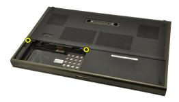
**4.** Press the rubber feet towards the rear of the system to disengage the bottom door.
