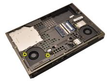
6. Remove the CPU fan from the system.
