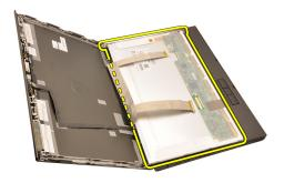
10. Remove the screws securing the display bracket to the display panel.
