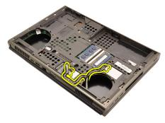
13. Loosen the four captive screws (1 > 2 > 3 > 4) on the heatsink.
