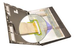
**8.** Peel back the adhesives and disconnect the RGB cable from the back of the display panel.
