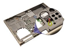
23. Disconnect the Bluetooth cable on the top side of the system board.
