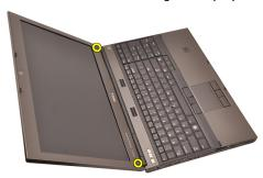
5. Carefully pry up the top edge of the display bezel.
