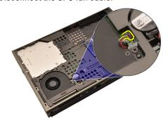
5. Remove the screws securing the CPU fan in place.
