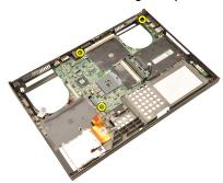
**28.** Gently lift the bottom edge of the system board assembly and raise it to a 20-degree angle.
