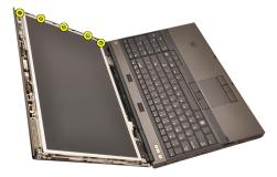
5. Remove the screws securing the display panel in place.
