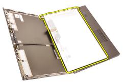
9. Remove the screws securing the display bracket to the display panel.
