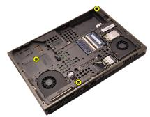
9. Loosen the captive screw at the bottom of the system.
