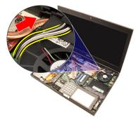
**14.** Loosen the captive screws securing the Low-voltage Differential Signaling (LVDS) cable in place.
