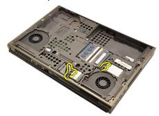
10. Remove the antennas from the routing channels.
