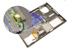
24. Disconnect the wireless switch cable.
