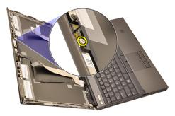
7. Lift and remove the camera and microphone module.
