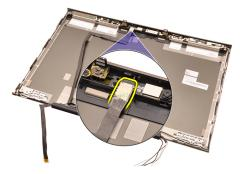
**15.** Pry up the camera cable from the display cover and remove the camera cable.
