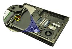
5. Remove the screws securing the graphics card fan in place.
