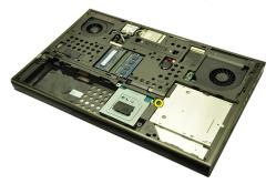
5. Remove the optical drive from the computer.
