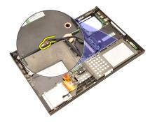
25. Remove the screws securing the hinge cover in place.
