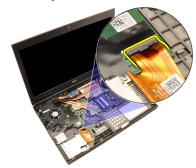
**10.** Remove the screws securing the ExpressCard module in place.
