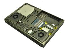
**5.** Remove the screw securing the hard drive latch in place.
