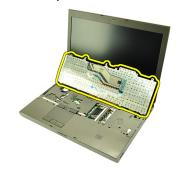
**8.** Peel back the adhesive tape securing the keyboard data cable to the back of the keyboard.
