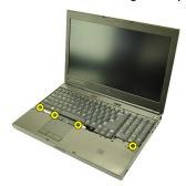
**5.** Starting from the bottom of the keyboard, separate the keyboard from the system and turn the keyboard over.
