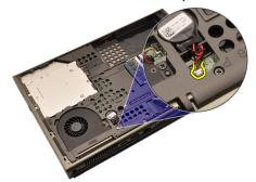
5. Pry up the coin—cell battery from the adhesive.
