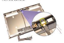
14. Pry up the LVDS and camera cable from the display cover.
