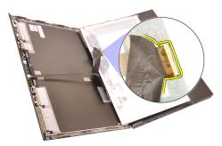
8. Remove the display panel from the display assembly.
