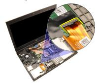
10. Remove the screws securing the Input/Output (I/O) board in place.
