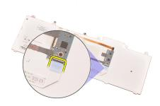
10. Peel the keyboard data cable away from the keyboard and remove.
