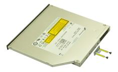
7. Remove the optical drive bracket from the drive.
