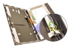
9. Remove the screws securing the digitizer in place.
