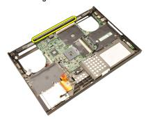
27. Remove the screws securing the system board in place.
