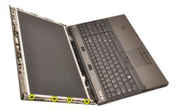
5. Remove the screws on the right side securing the display panel in place.
